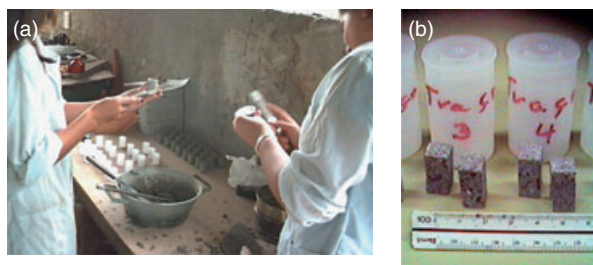
Figure 1 (a) Specimens of 30 mm diameter and 40 mm in height made with sieved concrete. (b) Tests samples of 10 \times 10 \times 20 mm used in mercury intrusion porosimetry tests.
