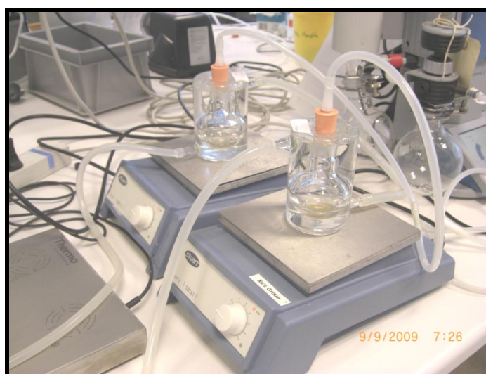
FIGURE 1 – Water-jacket reactors for interesterification reactions
