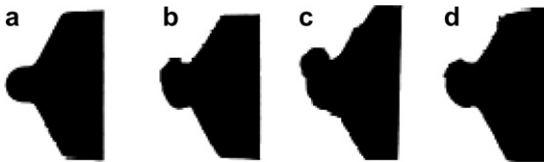
Fig. 4. Injector after EMA Engine test cycle-200 hours (ethyl canola): (a) clean injector; (b) B0; (c) B50; (d) B100 [22].
