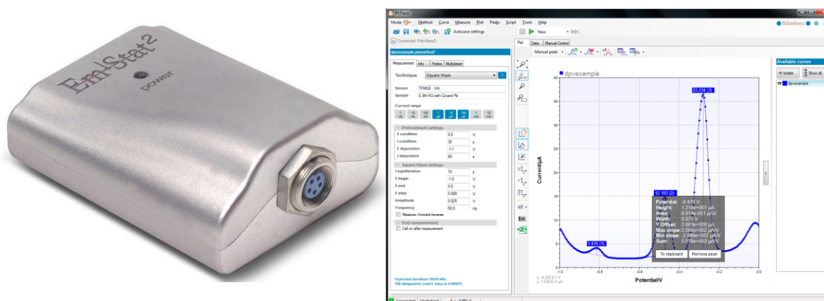
Figura 31 – Potenciostato PalmSens EmStat2 e a tela do software PsTrace.
